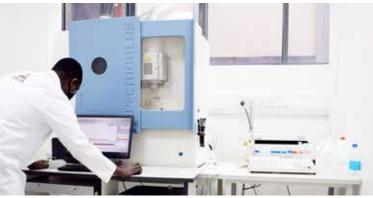
Induction Coupled Plasma Optical Emission Spectrometer ICP OES
